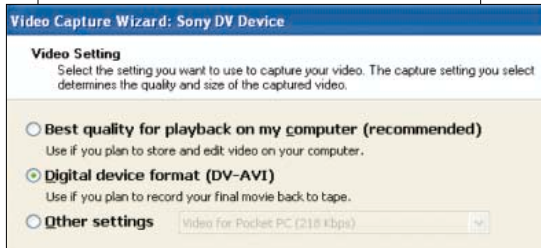
FIGURE 2: Capturing your video in DV format ensures the highest possible output quality.
