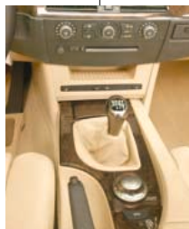
IDRIVE The BMW control knob replaces dozens of dashboard switches.
