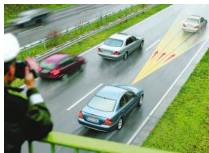
FOLLOW ME Mercedes-Benz radar maintains safe following distances.
