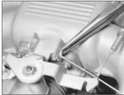
9.9 Pinch the plastic retainer, and push it through the bracket recess on the throttle valve
