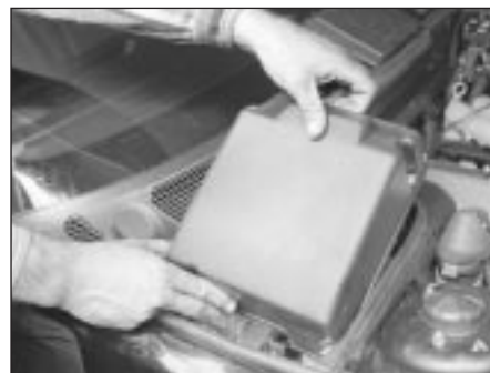
3.6c On all 1989 and later models, remove the four bolts and the protective cover to gain access to the fuel pump relay and ECU . . .
