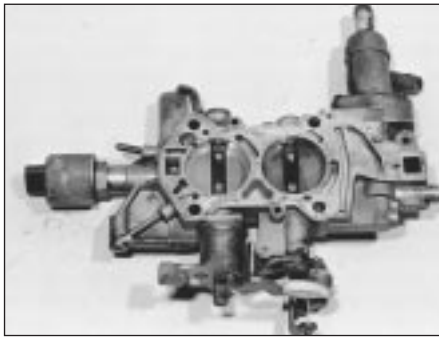
12.11a Throttle housing removed from the carburettor
