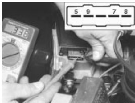
16.3 Connect an ohmmeter to terminals 7 and 8 of the airflow meter, and check for a smooth change in resistance as the vane door of the airflow meter is slowly opened and closed
