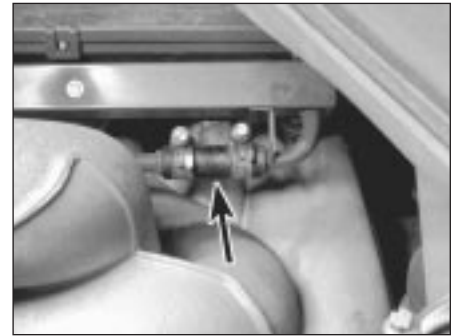
5.2 When checking the fuel lines, don't overlook these short sections of fuel hose attached to the main fuel rail - they're a common source of fuel leaks
