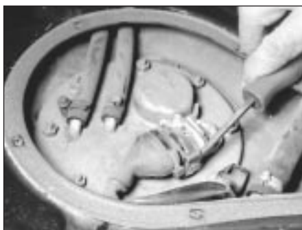
4.17b To unplug the connector, prise the bracket until the notch aligns with the slot on the retaining clip, and release the connector from the assembly
