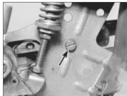
12.7 Throttle positioner bracket-to-throttle housing screw (arrowed)
