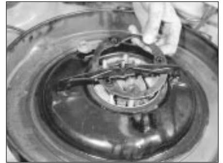
8.6b . . . and remove the metal ring
