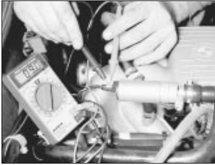
21.9 Check the resistance of the idle air stabiliser valve - it should typically be 9 to 10 ohms (L-Jetronic system)
