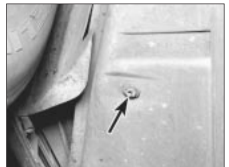
6.4 Remove the tank drain plug (arrowed) and drain the fuel into a suitable container
