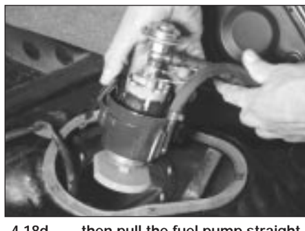
4.18d . . . then pull the fuel pump straight up and out of the turret at the bottom of the fuel tank (keep all the fuel lines intact)
