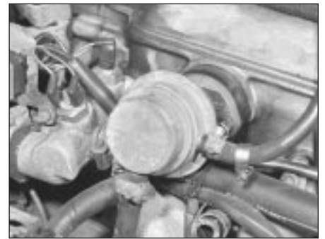
4.1 Fuel pump on carburettor engines
