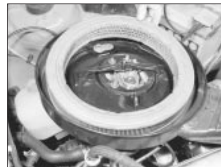
8.3 Remove the air cleaner element, and wipe clean the body and cover
