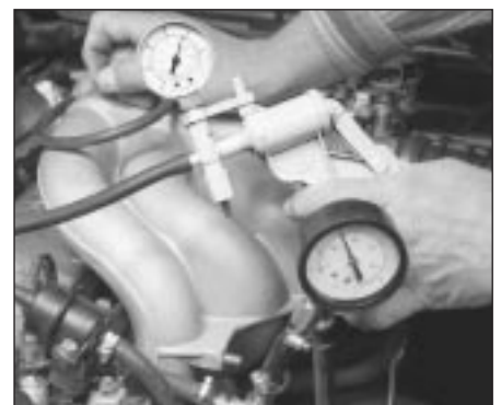
18.5 Carefully watch the fuel pressure gauge as vacuum is applied (fuel pressure should decrease as vacuum increases)
