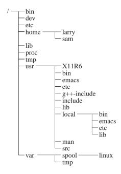
Figure 3.1: A typical (abridged) Linux directory tree.
