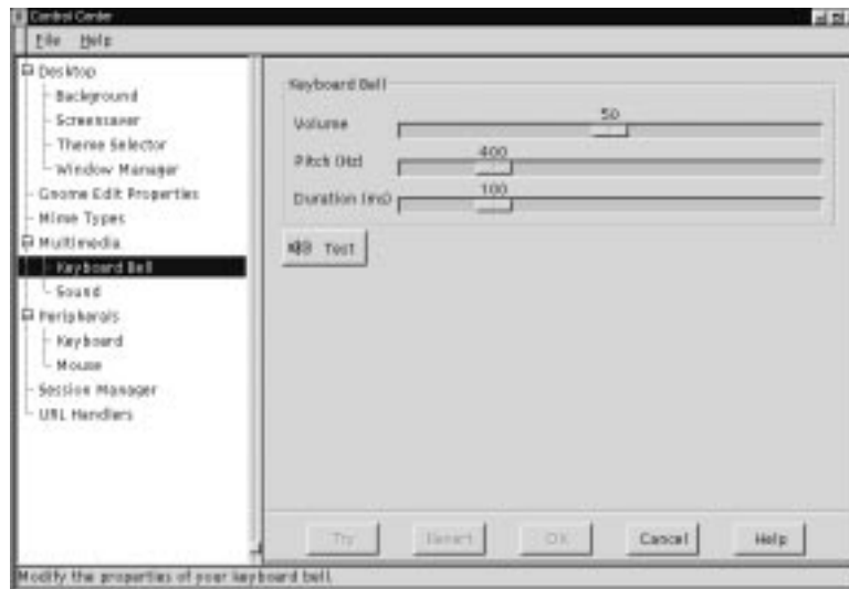
Figure 9-9. The Keyboard Bell Capplet
