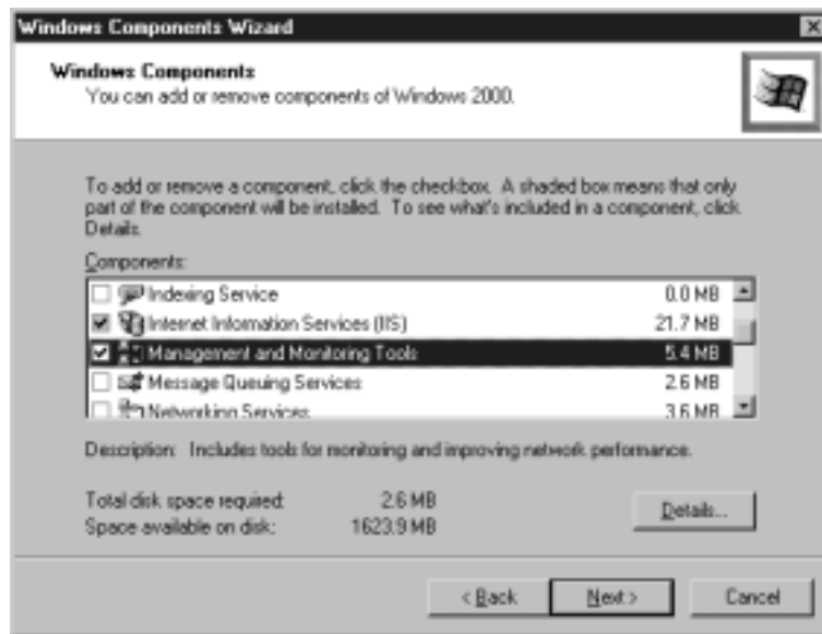
Figure 12.7 Preparing to remove a subcomponent of Management and Monitoring Tools.
