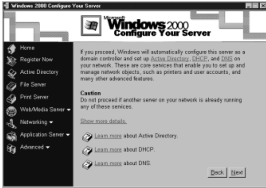
Figure 3.3 The Configure Your Server program will install Active Directory, DHCP, and DNS.
