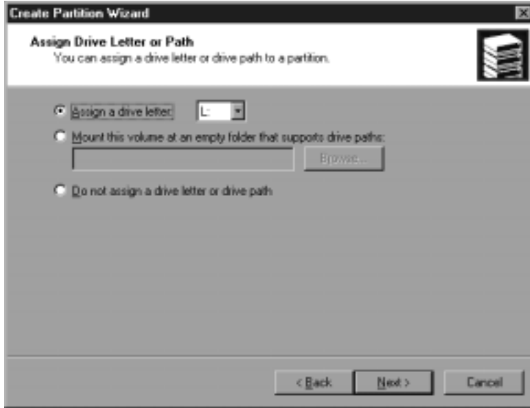
Figure 19.5 Selecting the drive letter, path, or neither to assign the new partition.
