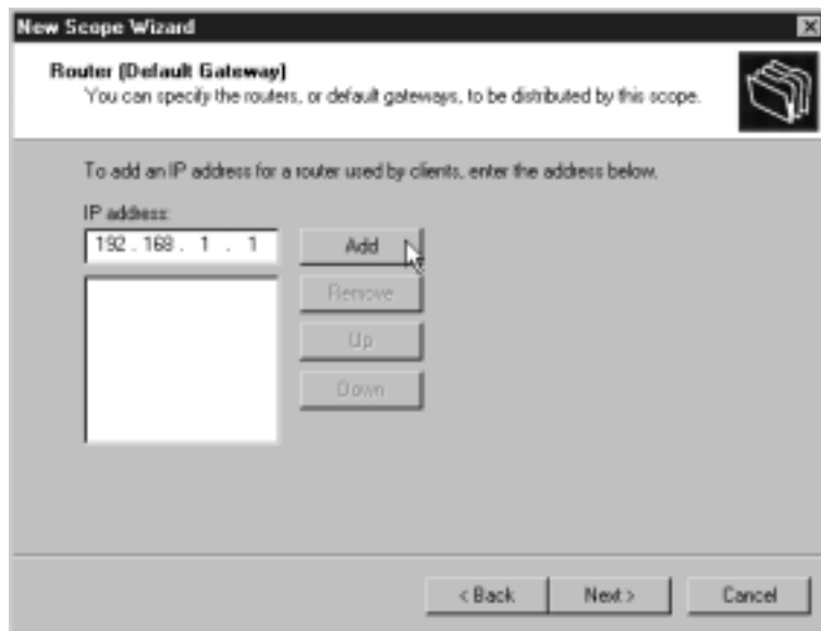
Figure 6.9 Specify one or more default gateways from the Router (Default Gateway) page.
