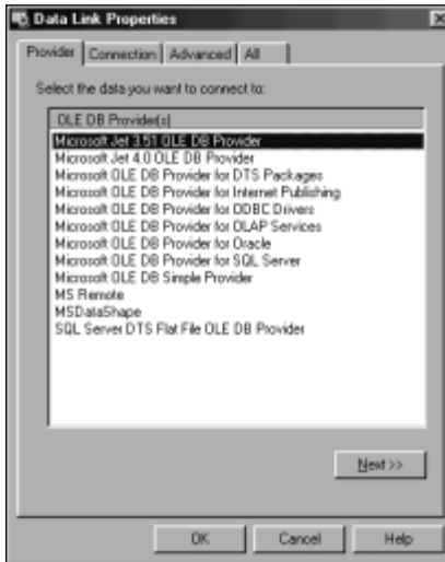
Figure 29-1: Choosing the proper OLE DB Jet provider.
