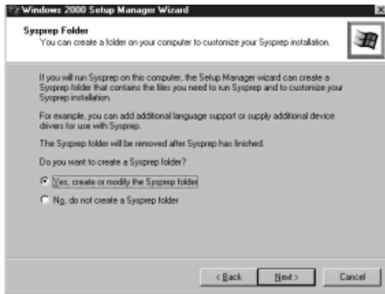
Figure 3.20 Select whether you want Setup Manager to create the Sysprep folder, or whether you will create it manually.
