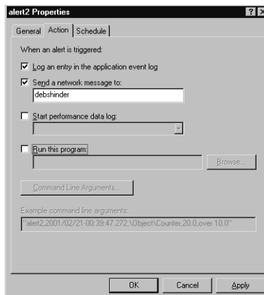
Figure 11.10 You Can Select One or More Actions to Be Taken When the Alert Is Triggered
