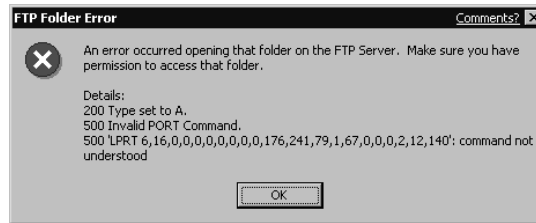
Figure 8.55 PORT Command Failure with FTP Filter Disabled
