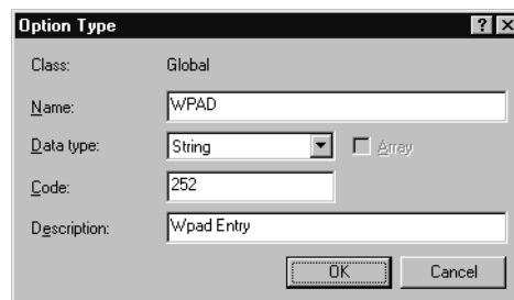
Figure 7.20 Adding a DHCP Option to Support Autodiscovery
