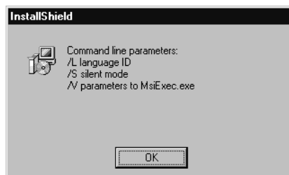
Figure 7.14 Command-Line Parameters for Client Setup
