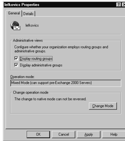
Figure 4.32 Displaying Administrative and Routing Groups in Exchange System Manager
