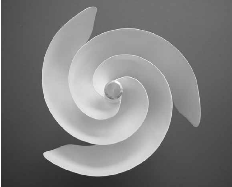
Figure 1.3 Mixer/impeller inspired by kelp (Rotor 7-03)
