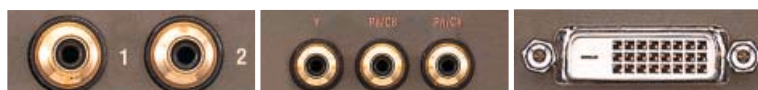
▲ Composite is a basic connection ▲ Component video sockets ▲ The latest TVs have DVI
