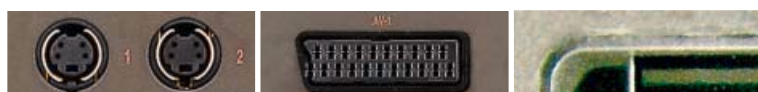
▲ S-video offers better quality ▲ Most TVs have SCART sockets ▲ HDMI carries video and sound
