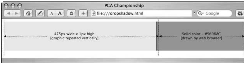
Figure 4-7: The container div with background graphic applied and viewed in a Web browser. Extra notation has been added to illustrate which area is an image and which area is drawn by the browser.
