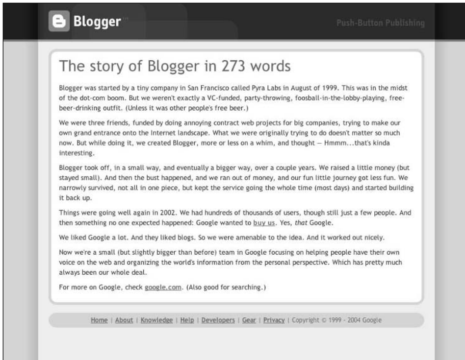
Figure 3-58: The result of setting no class attribute on <body>. Only <div id="main"> displays.
