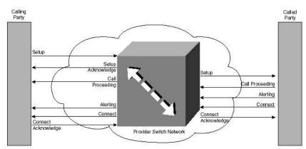
ITU-T Q.931 is specified as the protocol for Layer 3 of the D channel. The protocol messages and their rules for exchange are derived from the DSS1 protocol suite. And if you have the problem mentioned, you have probably configured the BRI settings wrong. Reference:
