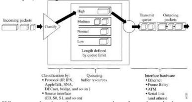
When a packet is to be sent out an interface, the priority queues on that interface are scanned for packets in descending order of priority. The high priority queue is scanned first, then the medium priority queue, and so on. The packet at the head of the highest queue is chosen for transmission. This procedure is repeated every time a packet is to be sent.
