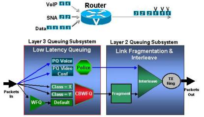
This method is more complex and flexible than IP RTP Priority. The choice between the methods should be based on the patterns of traffic in your real network and your actual needs.
