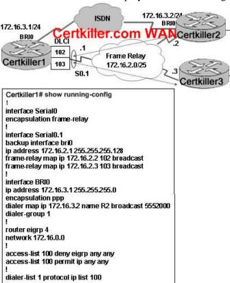
Certkiller 1 is connected with a multipoint subinterface over the Frame Relay to the spoke routers Certkiller 2 and Certkiller 3. The ISDN interface is configured to provide a back-up link should the primary connection to Certkiller 2 fail. However, when the PVC to Certkiller 2 drops, the BRI interface remains in "standby" mode and does not bring up the back-up link. Based on the information and the configuration file shown above, what could the problem be?
