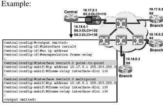
As this example shows, you should remove any network-layer address assigned to the physical interface. If the physical interface has an address, frames will not be received by the local subinterfaces. Although using layer 3 addresses on the main interface is not recommended, it is indeed possible to do this, therefore, B is correct in addition to C. Reference:
