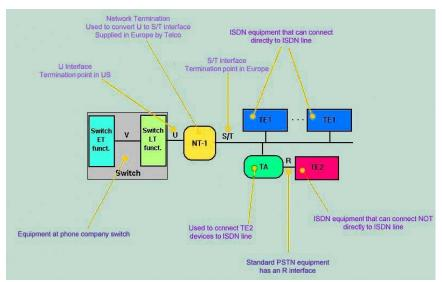
TA: Terminal Adaptor. This lets old, TE2 stuff talk to the ISDN network. It also adapts other kinds of equipment, like ethernet interfaces, to ISDN.
