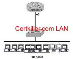
Each of the hosts is connected to their own 10Mbps half-duplex switch port to the e0 interface of a router. How much bandwidth is available to each individual host?
