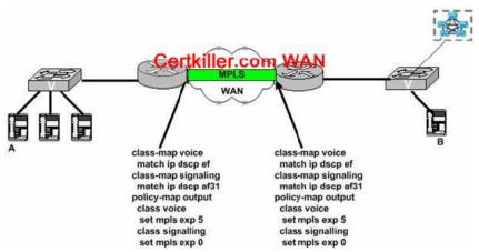
The LAN switches (and any other equipment in the cloud) do not mark or remark the packets. With regard to the QoS configuration in the exhibit, when IP Phone A calls IP Phone B, how will the voice and signalling packets be marked by the time they arrive at IP Phone B?
