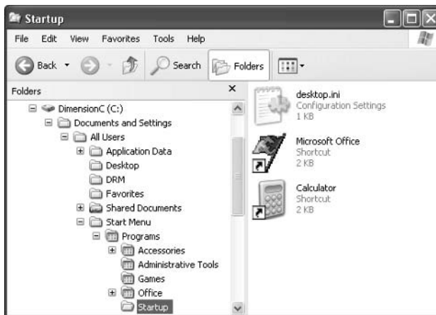
Figure 5-8: Put a shortcut to the Calculator in the \Startup folder, and it starts every time Windows does.
