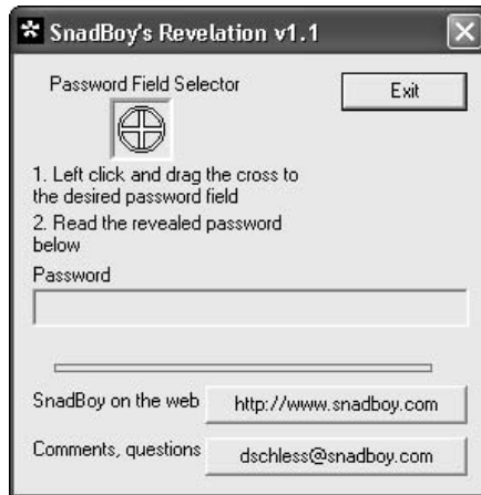
Figure 2-1: SnadBoy's Revelation lets you see passwords that appear as **** on the screen.
