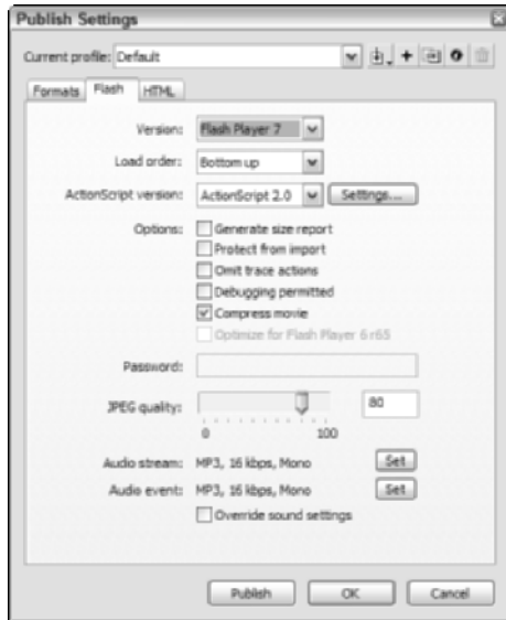
Figure 7-2: Use the Flash tab of the Publish Settings dialog box to set options for the SWF movie file.
