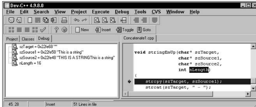
Figure 10-6: Setting a watch allows the programmer to monitor the value of a variable.
