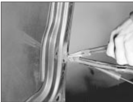
10.9 Pull off the clip with needle-nose pliers
