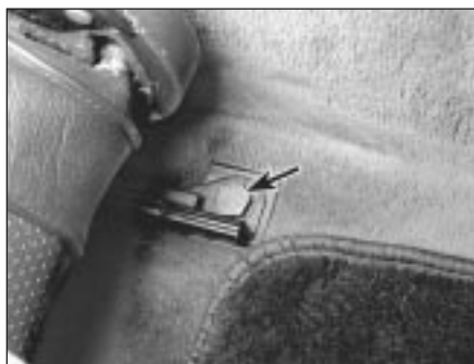
20.1 The front seats are held in place by bolts (arrowed)
