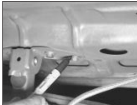
10.1 Use paint or a marking pen to mark on the hinge plate around the bolt heads - mark around the entire hinge plate, if desired, before adjusting the bonnet
