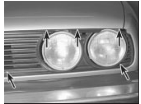
9.2b Side grille screw locations (arrowed)
