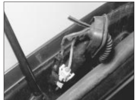
14.11 Removing the wiring from the rear pillar (5-Series)
