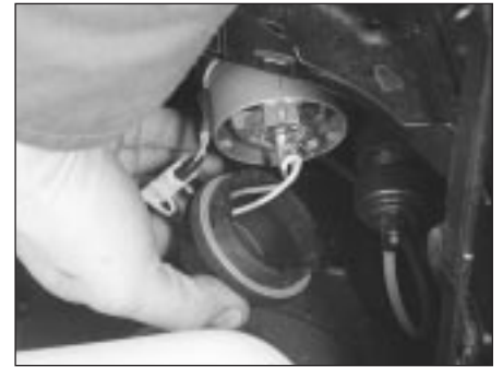
12.9 Twist and release the headlight inner cover
