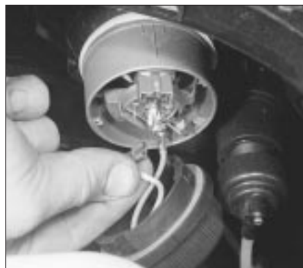
12.10 Disconnecting the wire from the rear of the headlight bulb
