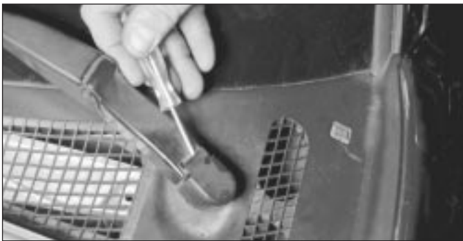
16.2a Use a small screwdriver to detach the wiper arm nut cover, or swivel the cover up
