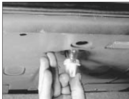
15.3b On models with high-mounted centre brake lights, the self-earthing holder is accessible from the luggage area - pull the holder out . . .
