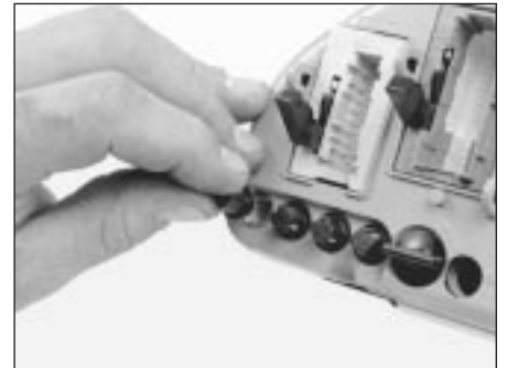
15.5 After removing the instrument cluster (see Section 10), turn the bulbholder anti-clockwise to remove the bulb
