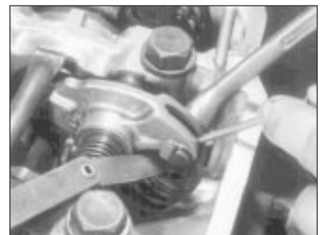
18.6 The valve clearance is adjusted by turning the eccentric with a wire hook - once the specified clearance is obtained, tighten the locknut with a spanner, then remove the feeler gauge
