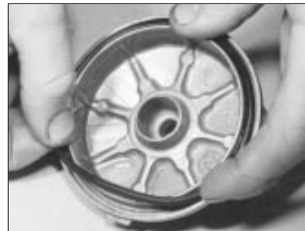
6.19 Renewing the rubber O-ring in the cover
