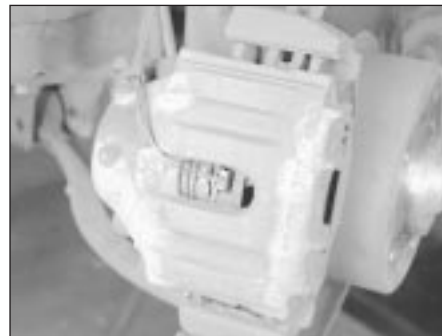
26.11 Look through the caliper inspection window to inspect the brake pads - the pad lining which rubs against the disc can also be inspected by looking through each end of the caliper
