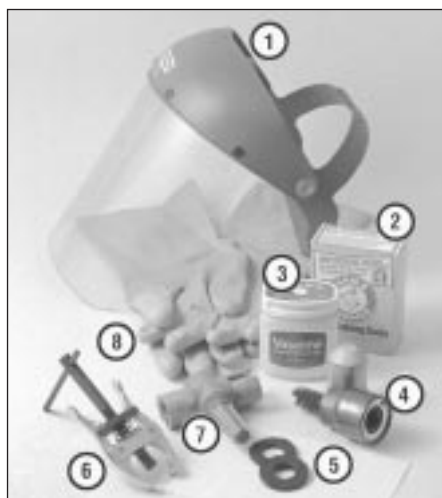
13.1 Tools and materials required for battery maintenance
