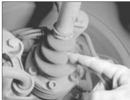
25.2 Gently probe the driveshaft boots to check for cracks
