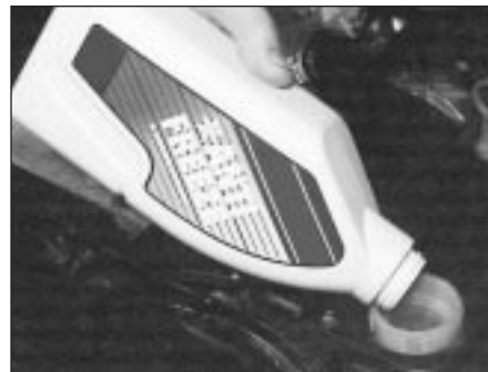
4.9d Adding antifreeze mixture
