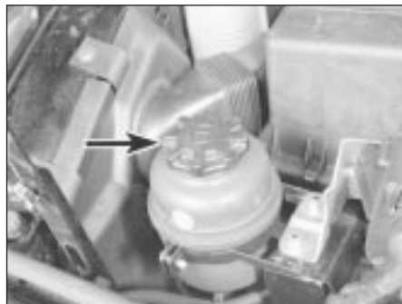
7.2 The power steering fluid reservoir (arrowed) is located on the left side of the engine compartment
