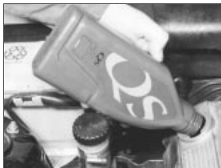
4.6b Topping-up the engine oil
