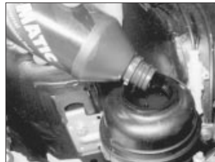
7.6 Adding fluid to the power steering reservoir
