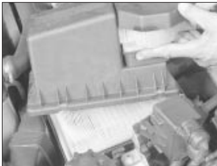
20.6a Rotate the cover upwards . . .
