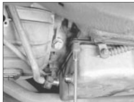
28.6 Use a socket and extension to remove the bolts and brackets
