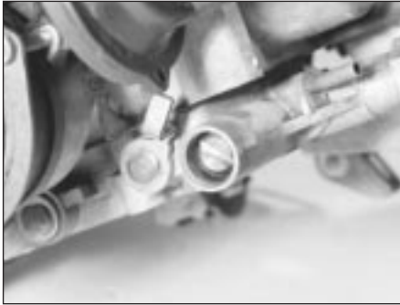
12.3 Idle speed adjustment screw on the 2B4 carburettor (shown with the carburettor removed)
