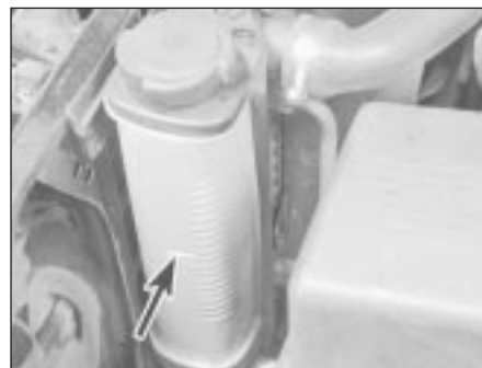
4.9a On some models, the expansion tank (coolant reservoir) is mounted on the radiator - make sure the level is kept at or near the FULL mark (arrowed)
