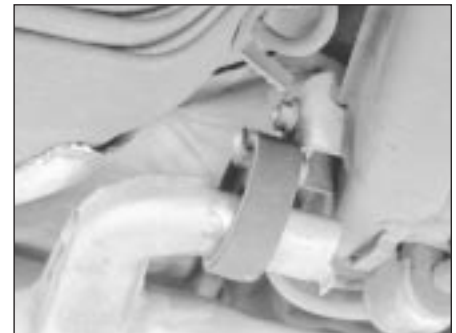
23.2 Check the exhaust system rubber mountings for cracks
