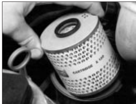
6.17c ... and lift out the cartridge
