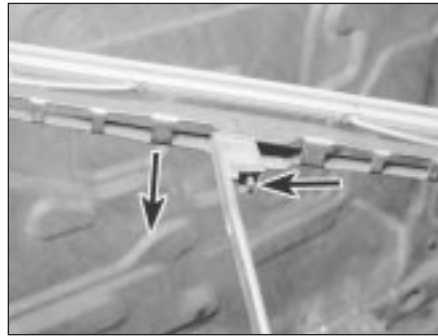
27.5 Press the retaining tab in, then slide the wiper blade assembly down and out of the hook in the end of the wiper arm
