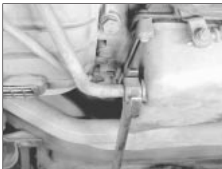
28.5a Unscrew the dipstick tube collar
